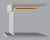
The low header model is used in underground parking and car parks, for example.
